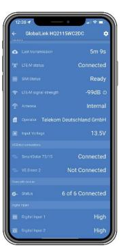
On the status screen there is information about the connectivity to the LTE-M network and the Victron Remote Management portal. For the device to work properly, the SIM status should be Ready and the LTE-M status must be Connected. You can also check if the correct antenna is selected and the current signal strength. The status screen also shows the operator name and number. It is not possible to select one yourself, even if more than one network is available in your region.
