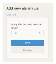
Note that the time set is the amount of time the high or low condition is active before an alarm is generated. It can then take an additional amount of time (up to 15 minutes) before that alarm is sent to VRM and email notification is sent.
